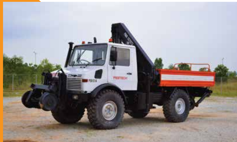
Road / Rail Tip Truck with 10t Crane /Man Bucket (Unimog) Mercedes Unimog - 9 Tons/m crane
