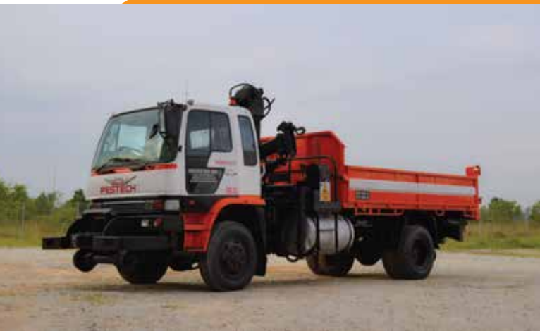
Road / Rail Tip Truck with 10t Crane/ Man Bucket 3 Way Tipper - Hiab 6 Ton/m crane
